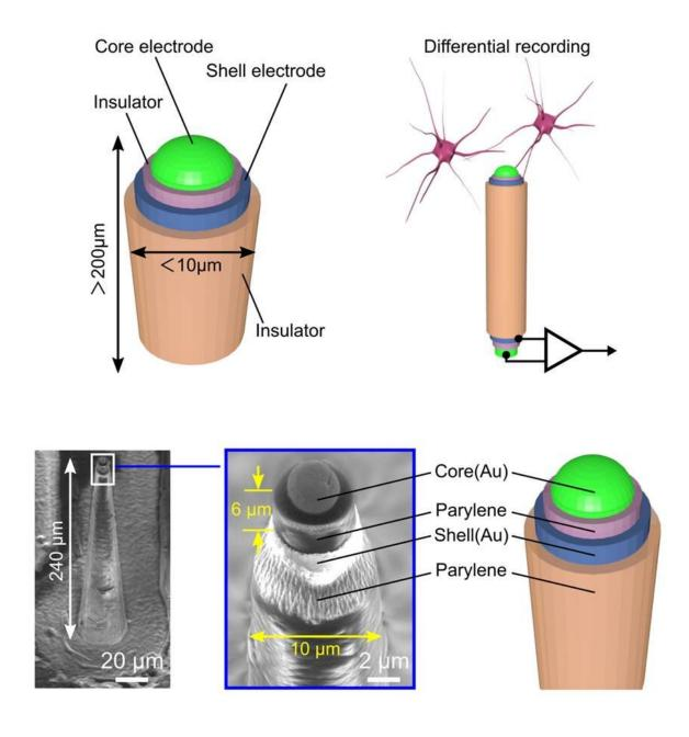
Local-differential recording of neuronal activities (top) Fabricated coaxial needle-electrode (bottom) Credit: Toyohashi University Of Technology.
