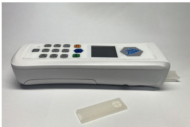
A prototype of the handheld ammonia blood detector and associated test strips, developed by researchers at Stanford. Credit: Thomas Veltman
