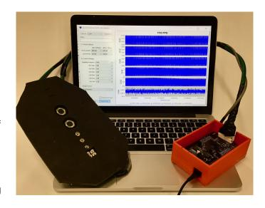
Prototype of the external fetal oxygen monitor developed by engineers at UC Davis. The device uses light to directly measure fetal oxygen saturation. Existing monitors used in the delivery room infer fetal oxygen by measuring fetal heart rate and contractions, and have a high false positive rate leading to many Cesarean sections. The new device has so far been successfully
