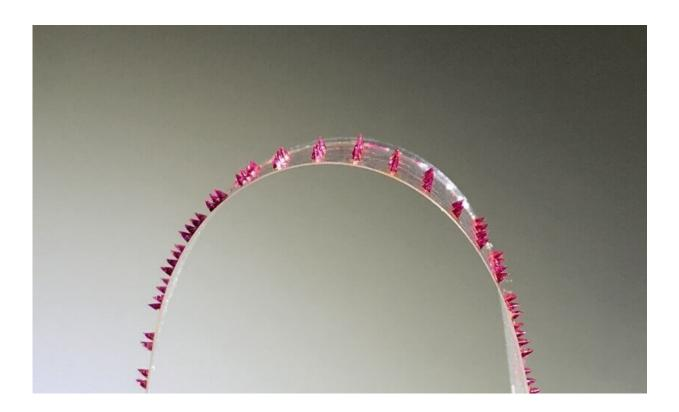
Microneedles, made of a biomaterial mixed with therapeutic agents, are attached to a strip of tape, needles facing down. The strip is applied to the wound area of the skin and the tape removed. The needles are embedded into the skin and degrade, delivering the therapeutic agent under the skin. Credit: Khademhosseini Lab
