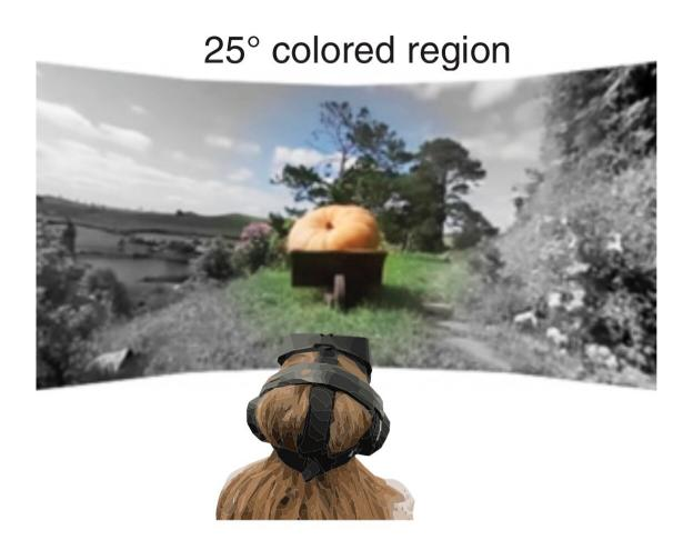
Gaze contingent rendering in immersive virtual reality. Observers wore a virtual reality headset equipped with real-time binocular eye trackers. As observers explored a scene, areas of the visual environment were desaturated so that only the area where they were looking was in the color. Participants were often unaware when up to 95 percent of their visual field was desaturated during this
