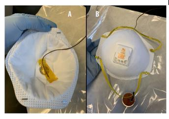
Inner and outer view of an N95 mask between dry heat treatment cycles showing no deformation of the respirator. A thermocouple is affixed to the inner surface of the respirator with Kapton tape to measure the surface temperature of the mask over 10 heating cycles in a standard laboratory convection box oven. Masks are heat treated inside a self-sealing autoclave pouch (background) to prevent dispersion of viral particles from airflow inside the oven. Credit: Trevis Massey/LLNL
