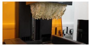
The valves being manufactured in a 3D printing machine at the University of Leeds. Credit: University of Leeds
