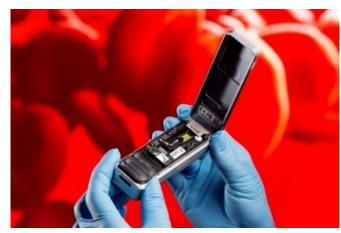
Nanopore sequencer used for real-time microbial cellfree DNA analyses in septic patients. Credit: Fraunhofer IGBI
