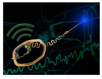
Recording the activity of individual neurons is made possible by this tiny, wireless, battery-free device. Credit: University of Arizona Gutruf Lab
