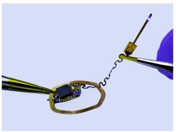
Recording the activity of individual neurons is made possible by this tiny, wireless, battery-free device. Credit: University of Arizona Gutruf Lab
