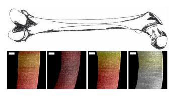
Researchers used a new endoscopic OCT system to visualize variances in pig cartilage thickness. The image shows a sketch of a femur and processed OCT images with thin regions shown in dark red and thicker regions more yellow and white. Scale bar is 250 microns. Credit: Evan T. Jelly, Duke University
