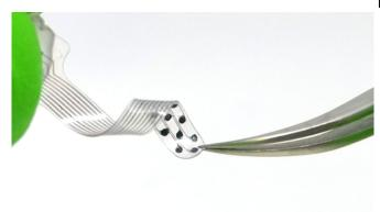
The highly elastic implant conforms neatly to the curved surface of the auditory brainstem and can therefore send highly targeted electrical signals. Credit: EPFL
