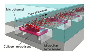
This diagram demonstrates how the engineered tissue model works to mimic the clotting upon blood vessel injury. Platelets adhere to the collagen microtissue that represents the collagen layer in the blood vessel. The micropillars that support the microtissue sense the stiffness of the microclots that form when exposed to different flow rates, which mimic venous or arterial flow in the body.? Credit: Zhao, Neelamegham, et al/Nature Communications
