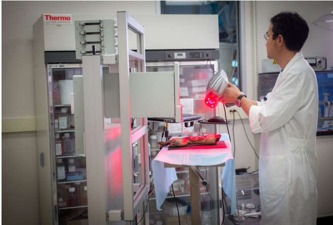
A WFIRM technician operates the mobile bio printer for skin printing on a limb demo. Credit: WFIRM
