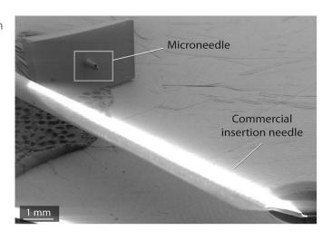
The microneedle is significantly smaller than the commercial standard for continuous glucose monitoring. Credit: KTH
