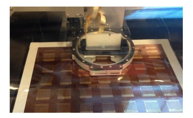
An inkjet printer layers gold nanoparticle ink constructing a batch of biosensors capable of forming the detection platform for a breast cancer protein in blood. The printer can be observed in this video depositing ink in a specific pattern to construct the sensor chip. Credit: Colleen E. Krause
