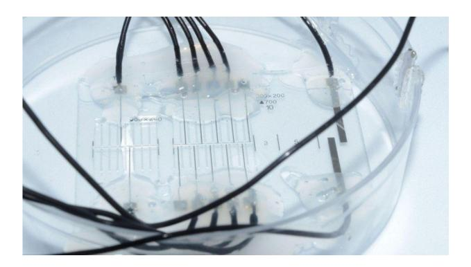
The "nerve-on-a-chip" platform paves the way to using chips to improve neuroprosthetic designs. Credit: Florent-Valéry Cohen
