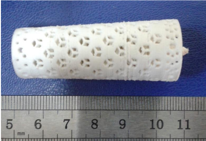
TPU bioresorbable composite implants for testing at the Ilizarov Center. Credit: Tomsk Polytechnic University (TPU)
