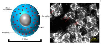
An oxygen nanobubble structure (left) showing gaseous oxygen core surrounded by cellulosic encapsulation. The oxygen nanobubbles can easily enter into tumor cells and can be visualized using ultrasound or dark field microscopy (right). Credit: Purdue University
