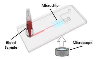
The AR-Chip quantitatively analyzes thrombus formation in blood flow. The microscope is used to inspect developing thrombi. Credit: Dr. Masanobu Ishii and Associate Professor Koichi Kaikita
