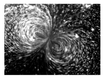
Cavitation microstreaming generated by a SonoVue microbubble and marked by fluorescent beads. Under ultrasound exposure, microbubbles can produce streaming flows which may contribute to blood-brain barrier opening and will be investigated directly using our in vitro platform. Credit: Miles M. Aron, courtesy of BUBBL, University of Oxford, England
