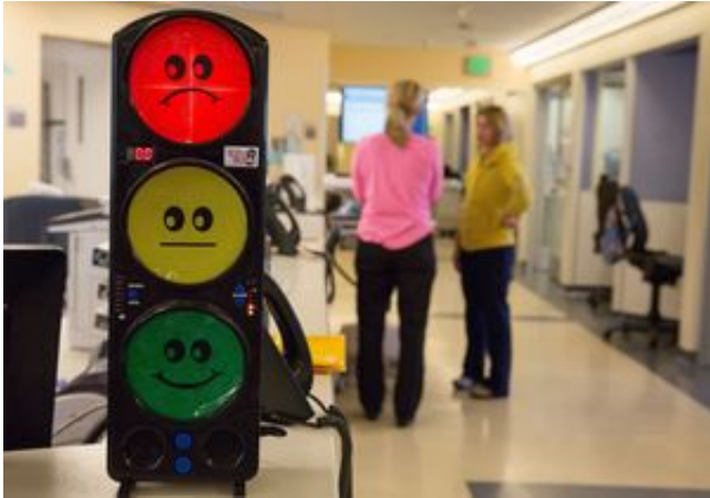
A stoplight noise monitor warns the staff at Mattel Children's Hospital UCLA when there's too much noise being generated. Credit: Reed Hutchinson/UCLA
