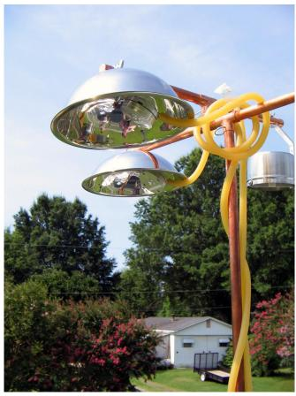
Air pollution monitors were deployed in more than 1,500 locations within the six different metro areas. In addition to air pollution data from state and local air agencies, these MESA Air monitors collected and measured variable levels of PM2.5, oxides of nitrogen, and black carbon, among other pollutants over two-week periods between 2005-2009. Credit: MESA-Air
