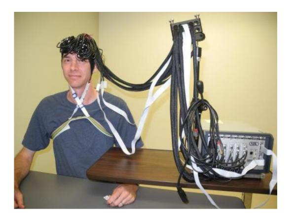
Dr. Wylie of Kessler Foundation demonstrates the portable device for recording functional near infrared spectroscopy in cognitive research studies of brain activation (NIRScout, NIRx Medical Technologies, LLC). Credit: Kessler Foundation
