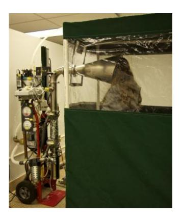
The Gesundheit II machine collects the breath exhaled from flu sufferers. Study volunteers sit for 30 minutes with their heads in the horizontal cone attached to the machine, which sucks in the air around their heads to collect tiny airborne droplets generated deep in the lungs. Researchers can then analyze the aerosols for the presence and quantity of virus. Credit: Donald Milton
