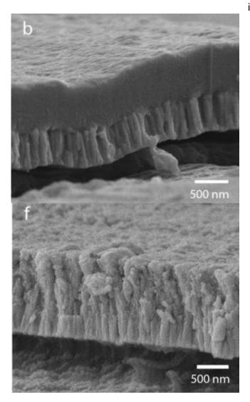
The top scanning electron microscope image (b) shows a cross section of the bioactive hydroxyapatite/YSZ coating without heat treatment. Note how the two layers are distinct. The bottom image (f) shows the coating after heat treatment. Note how the layers are now integrated.
