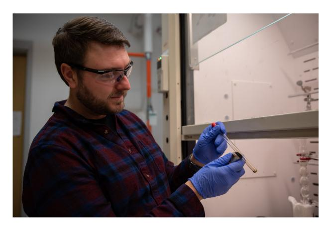
NIST researcher Sam Oberdick explored contrasts agents for MRI machines along with his cohort. His group tested iron oxide nanoparticles at lower-strength magnetic fields. These nanoparticles inside the liquid solution (pictured here) are magnetic and are pulled toward the magnet through a combination of magnetic
