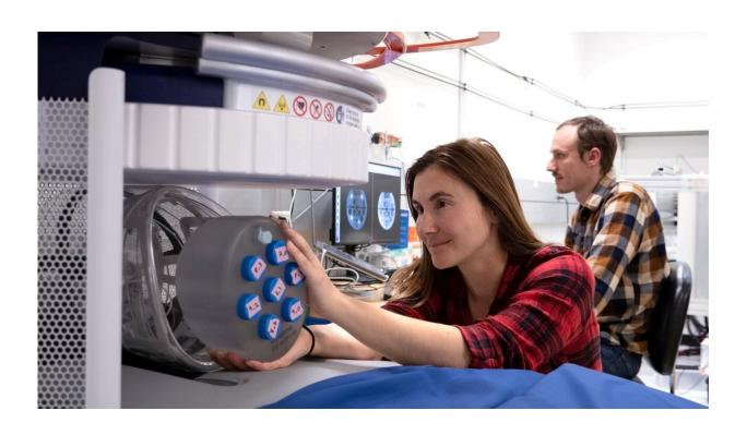
NIST researchers Kalina Jordanova and Stephen Ogier conduct MRI measurements using a magnetic field strength of 64 millitesla (mT), which is at least 20 times lower than the magnetic field in conventional MRI scanners, used for example in hospital settings. Credit: R. Jacobson/NIST
