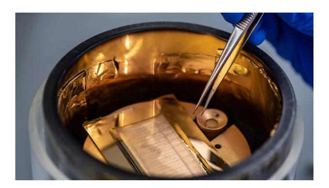
For the conductive structures, a thin layer of gold is deposited onto the 3D printed structure under high vacuum. Credit: Andreas Heddergott / TUM
