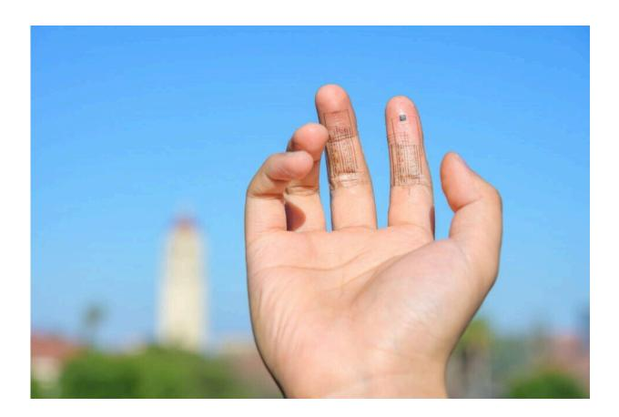
The e-skin is soft and stretchable, while also being able to mimic sense of touch and run efficiently at a low voltage. Credit: Jiancheng Lai and Weichen Wang of Bao Research Group at Stanford University
