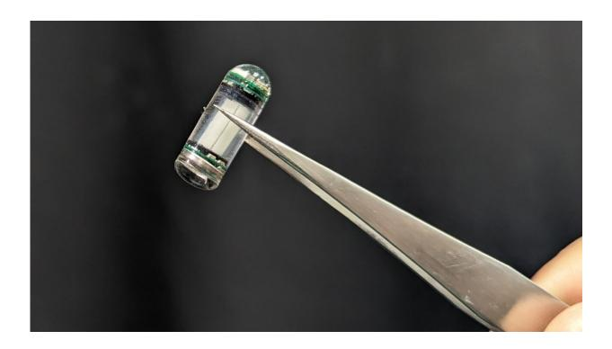
The components of the dosimeter fit into an 18mm by 7mm capsule, a common size for many supplements and medicines. Credit: National University of Singapore
