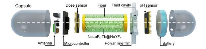
The components of the dosimeter fit into an 18mm by 7mm capsule, a common size for many supplements and medicines. Credit: National University of Singapore
