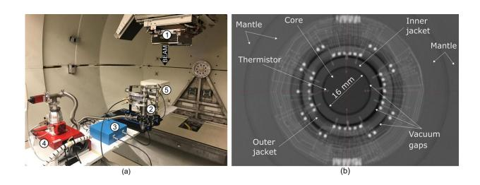
Experimental setup mounted on the patient couch and radiograph of the NPL PSPC. (a) (1) Gantry, (2) NPL PSPC, (3) measurement instrumentation for the NPL PSPC, (4) vacuum pump, (5) ionization chamber setup. (b) Radiograph of the front view of the NPL PSPC. Credit: *Scientific Reports* (2023). DOI: 10.1038/s41598-023-28192-0
