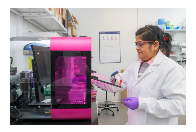
University of Delaware post-doctoral researcher Lina Pradham loads a protocol and plate into a bioprinter made by Inventia. Called the RASTRUM, the Inventia bioprinter prints synthetic matrices loaded with cells of interest into multi-well plates for 3D cultures that allow researchers to study mechanisms and screening of therapeutics. Credit: Evan Krape/University of Delaware
