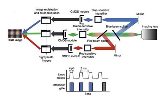
A three-channel camera separates Cherenkov emissions into red, green, and blue channels, allowing the investigation of the impact of variations in melanin and blood levels on the signal. This approach uses time-gated intensified cameras on all three channels to capture near single photon level images in each of the red, green, and blue wavelengths coming from the tissue. Credit: *Journal of Biomedical Optics* (2023). DOI: 10.1117/1.JBO.28.3.036005
