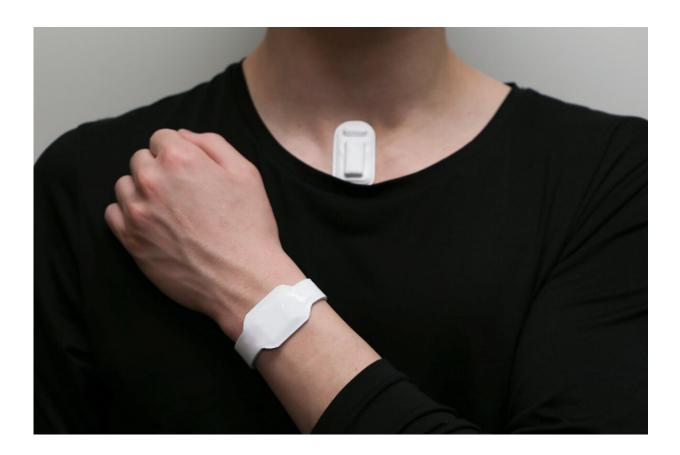
Developed by biomedical engineers and opera singers, the small, soft, flexible, wireless device sits on upper chest to monitor vocal activity in real time. When the user nears their vocal budget, an accompanying haptic device (located on the risk) vibrates an alert. Credit: Northwestern University
