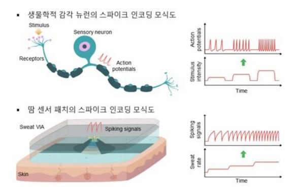
Schematic diagram of spike encoding in response to external stimuli by a biological sensory neuron and by the newly developed sweat sensor patch. Credit: Korea Institute of Science and Technology
