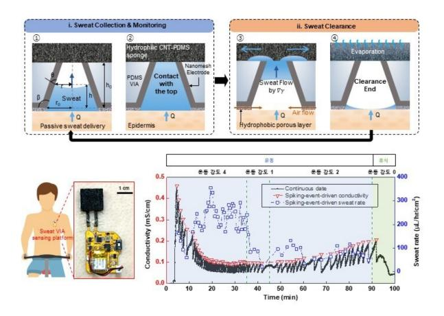
Structure and operating principle of the newly developed sweat sensor patch (top). Spike event-based wireless sweat monitoring clinical study using sweat sensor patch (bottom). Credit: Korea Institute of Science and Technology
