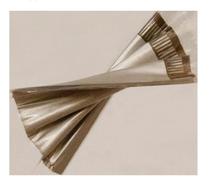
The wearable ultrasound sensor is flexible, allowing it to provide a continuous recording of cardiac activities before, during and after exercise or movement. Credit: Xu Laboratory at UC San Diego
