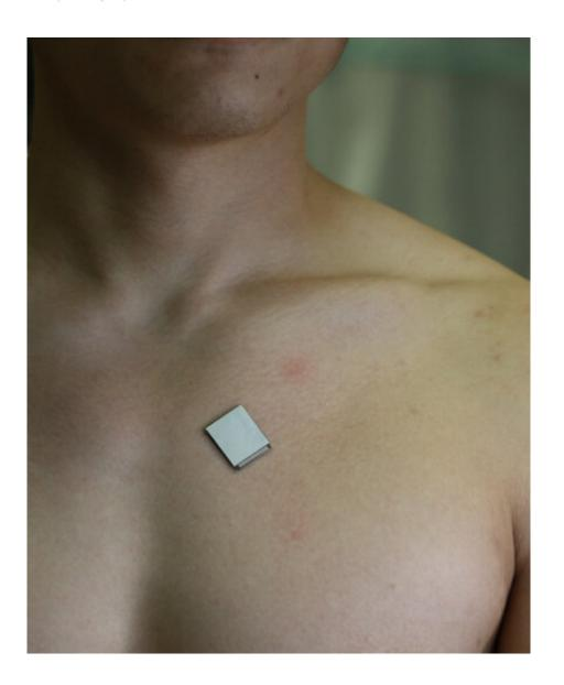
The wearable ultrasound sensor is roughly the size of a postage stamp, can be worn for up to 24 hours, and works even during strenuous exercise. Credit: Xu Laboratory, UC San Diego Jacobs School of Engineering
