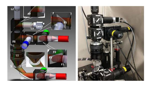
Researchers developed a portable and low-cost macroscopic mapping system for all-optical cardiac electrophysiology with applications in drug development and personalized treatments. (a) Schematic of the imaging system. (b) The actual setup. Credit: Heinson, Han, and Entcheva, doi 10.1117/1.JBO.28.1.016001.
