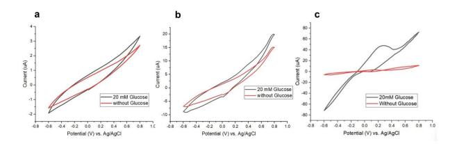
Glucose detection in 1X PBS solution using CV measurement for different
