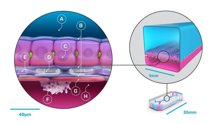
Schematic of the Emulate Liver-Chip. This diagram shows primary human hepatocytes (C) that are sandwiched within an extracellular matrix (B) on a porous membrane (D) within the upper parenchymal channel (A), while human liver sinusoidal endothelial cells (G), Kupffer cells (F), and stellate cells (E) are cultured on the opposite side of the membrane in the lower vascular channel (H). Credit: *Communications Medicine* (2022). DOI: 10.1038/s43856-022-00209-1
