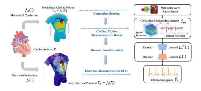
Working principle of contactless ECG monitoring. Credit: JIN Bochen et al.
