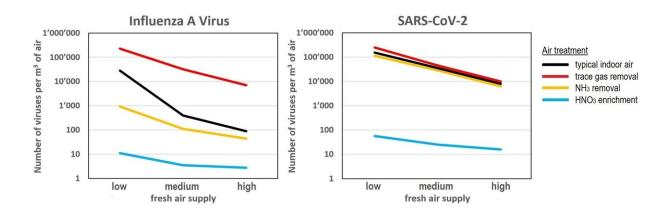
Concentration of infectious viruses in a room with one sick person per 10 m<sup>3</sup> as a function of the strength of fresh air supply with different types of air treatment with respect to nitric acid (HNO<sub>3</sub>) and ammonia (NH<sub>3</sub>). Credit: *Environmental Science & Technology* (2022). DOI: 10.1021/acs.est.2c05777
