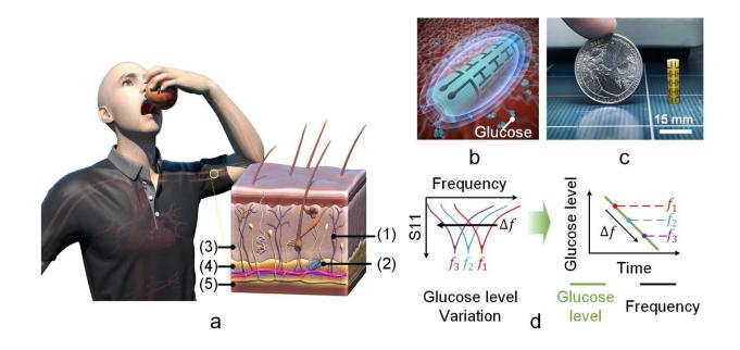
EM-based subcutaneous implant glucose sensor. (a) Illustration of EM-based implantable sensor for BGL tracking; (1) blood capillary (2) electromagnetic sensor (3) dermis (4) subcutaneous fat (5) muscle tissue. (b) Proposed implant sensor. (c) Sensor size (15 mm × 4 mm Ø) compared with a coin. (d) Sensor frequency trend and corresponding variations in BGL. Credit: UNIST
