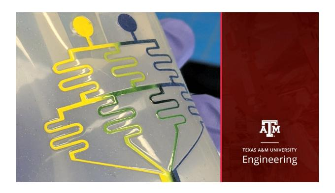
Laminated paper can direct fluid through porous paper structures with high accuracy and precision and can be used in complex fluid handling systems such as polymerase chain reaction COVID-19 tests and DNA sequencing machines. Credit: Texas A&M Engineering
