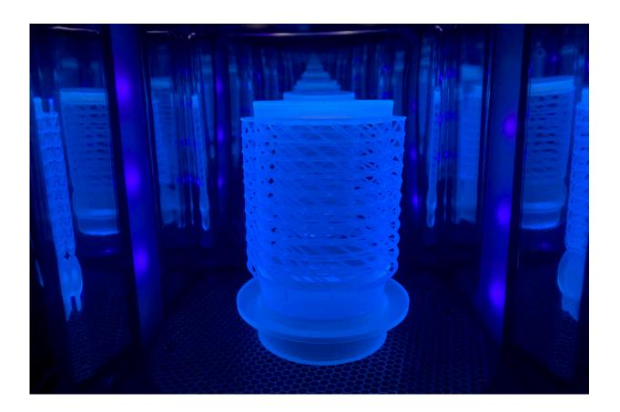
A large-scale replica of the scaffold that supports the heart tissue. In the miniPUMP, the scaffold is tiny—with many parts measured in microns. At such a fine scale, ordinarily stiff materials become flexible. Credit: Christos Michas, Alice White's lab at Boston University
