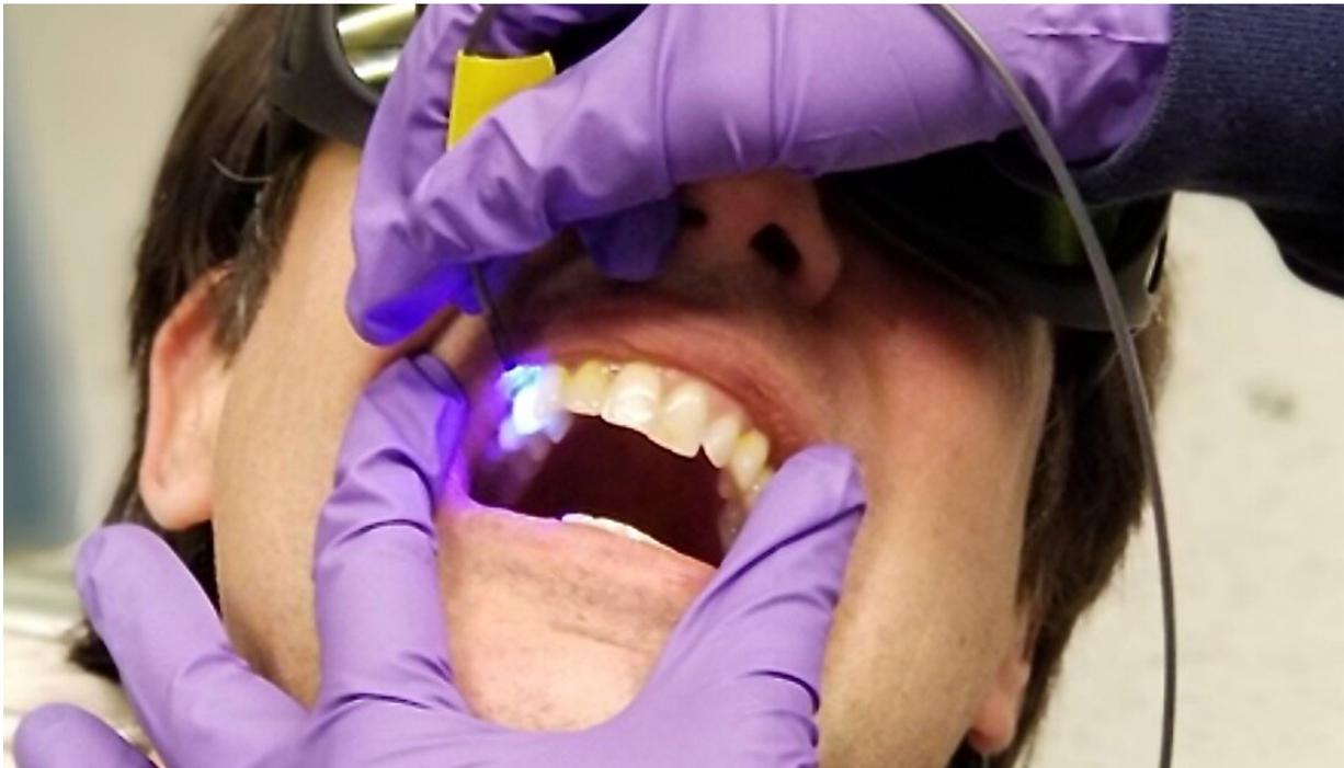
A new University of Washington dental tool prototype uses a low-power light system to monitor reactions with a fluorescent dye solution to find where tooth enamel is most at risk from the acidity of plaque. Credit: University of Washington and IEEE Xplore/Creative Commons
