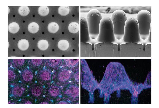
Bioengineered organoids with an in vivo–like tissue architecture. Top row: Scanning electron microscopy images of a polymer template used for fabricating hydrogel substrates with a realistic crypt-villus architecture (top and side views, respectively). Bottom row: 3D reconstruction of immunofluorescence images showing an intestinal tissue with realistic crypt and villi – "peaks and valleys" – anatomy of the real organ. Credit: Mike Nikolaev (EPFL)
