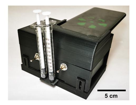
The microfluidic cartridge can be inserted into a portable device that also has a cradle for a smartphone, so the phone's camera can read the test results. Credit: Bill King, University of Illinois
