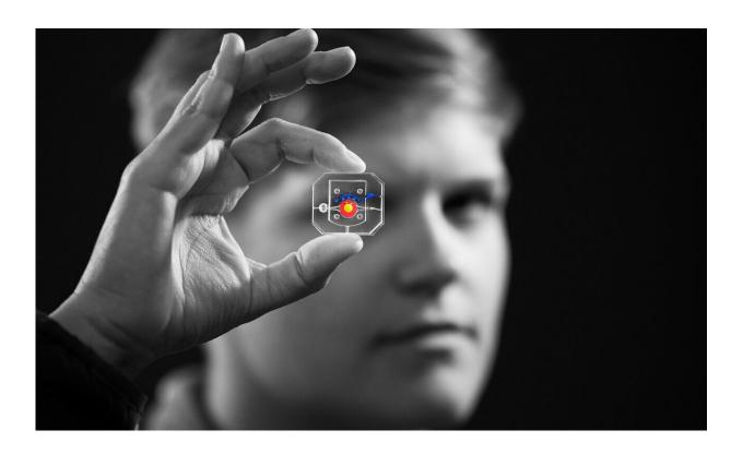
Rachel Young, a graduate student in Huh's lab, holds up their new eye-on-a-chip device. The latest iteration of the lab's eye-on-a-chip has a mechanical eyelid to simulate blinking, and was used to test an experimental drug for dry eye disease. By incorporating human cells into an engineered scaffolding, the eye-on-a-chip has many of the benefits of testing on living subjects, while minimizing risks and ethical concerns. Credit: University of Pennsylvania
