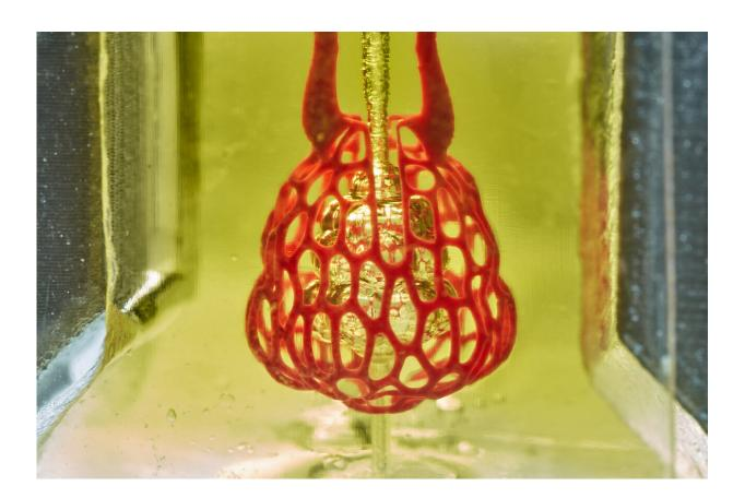
Bioprinting research from the lab of Rice University bioengineer Jordan Miller featured a visually stunning proof-of-principle -- a scale-model of a lungmimicking air sac with airways and blood vessels that never touch yet still provide oxygen to red blood cells. Credit: Jordan Miller/Rice University
