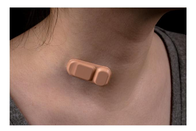
A woman wears this soft and flexible groundbreaking new sensor, developed by the Rogers Research Group at Northwestern University, which uses measurements of temperature and heat transfer to non-invasively tell if and how much fluid is flowing through a shunt in a hydrocephalus patient. In the study, the skin sensor allowed hydrocephalus patients to see within five minutes of placing it on their skin if there was flow through their shunt. Credit: Northwestern University
